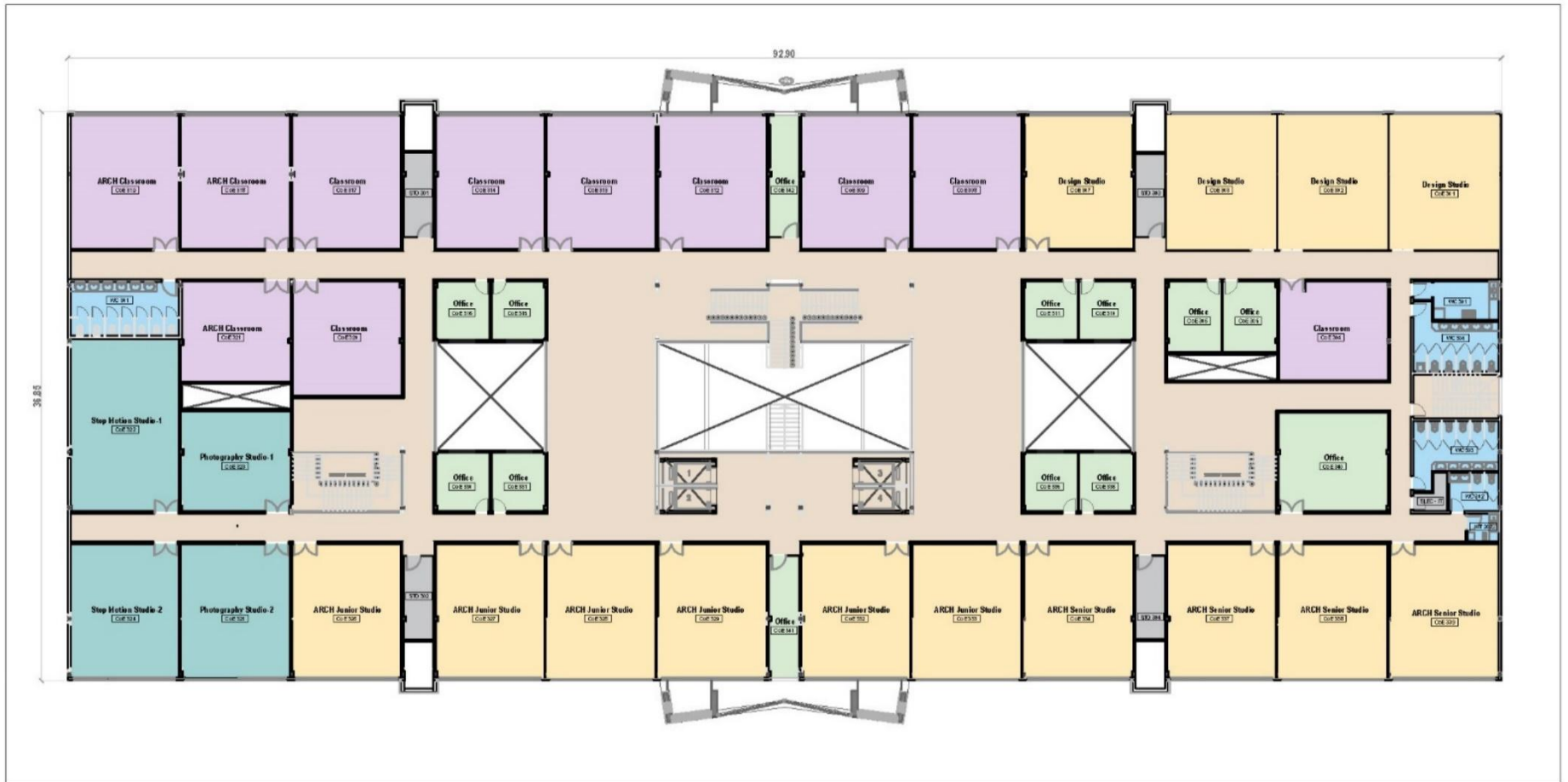
Fig. (16): The First Floor Plan for the CoE Building showing classrooms and Studios
