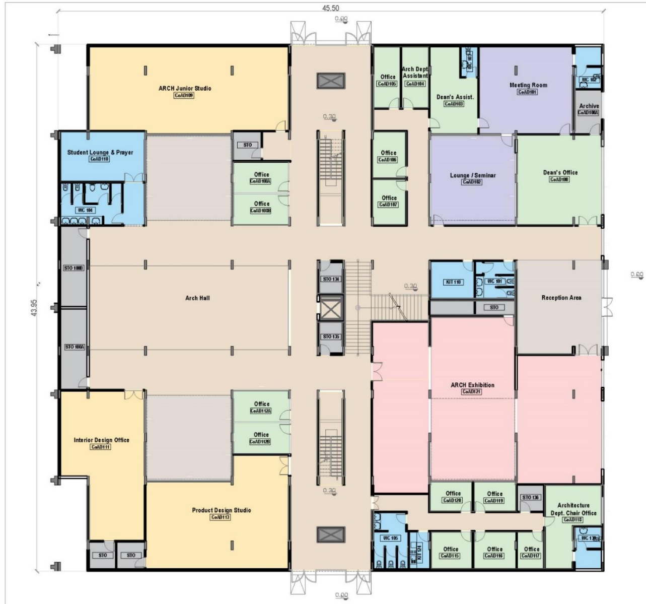
Fig. (14): The Ground Floor Plan for the CoAD Building showing classrooms and Studios
